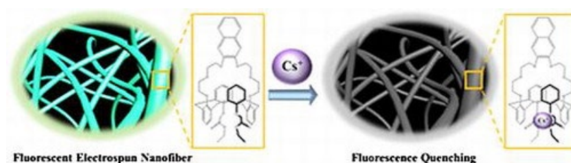
Figure 65 Nanofibrous embedded with fluorescent sensible calix[4]arene cesium probe (Ref. 164)
